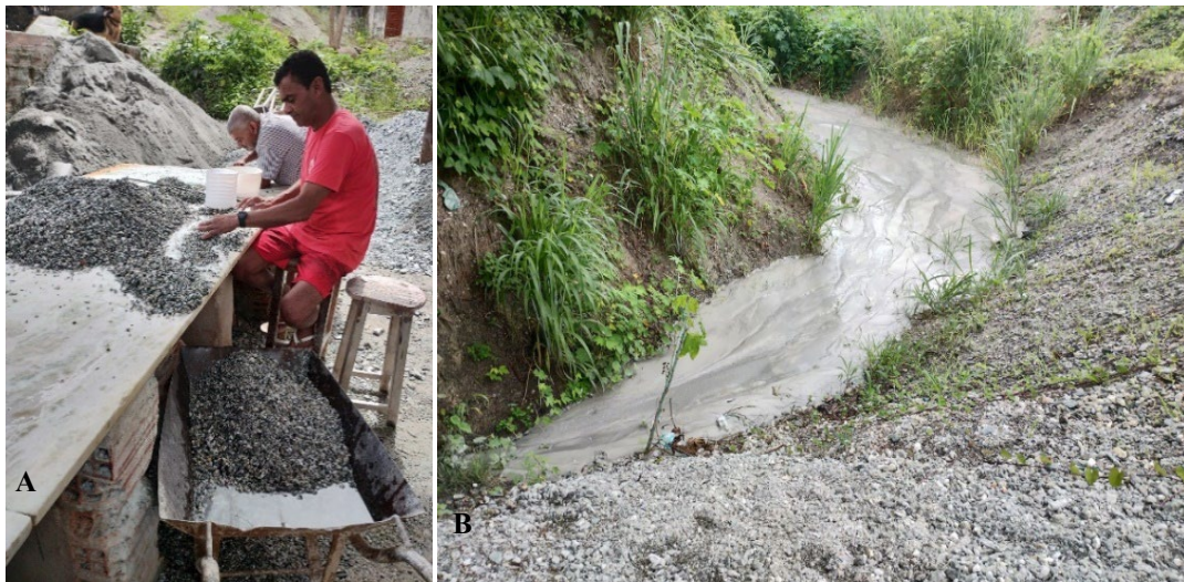
Figure 2: Manual recovery of emerald gemstones during the beneficiation process (A), and nearby silted watercourse (B). (Source: the author himself).
