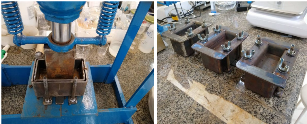
Figure 6: Compression device (left) and the finished test specimens (right). Source (the author himself).
