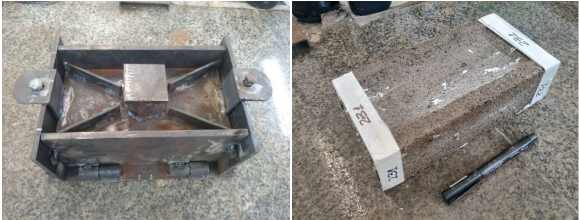
Figure 7: Metallic mold (left) and representative cement-free composite brick manufactured with polyester fabric waste (right). (source: the author himself).
