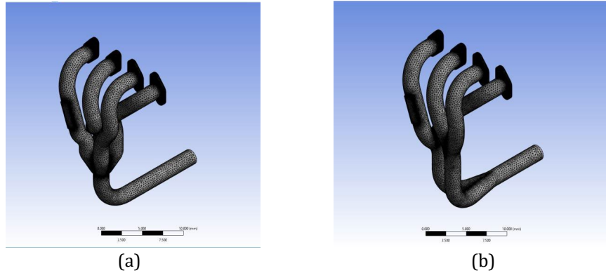
Figure 2: The Exhaust Manifold Meshing Image (a) 4-1 Exhaust Manifold and (b) 4-2-1 Exhaust Manifold.
