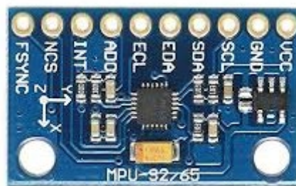
Figure 1: MPU-9250 nine-axis inertial measurement unit integrating a three-axis gyroscope, accelerometer, and magnetometer.
