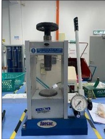
Figure 3: Manual hydraulic pellet press.
