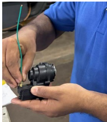
Figure 2: Manual panel pins insertion.
