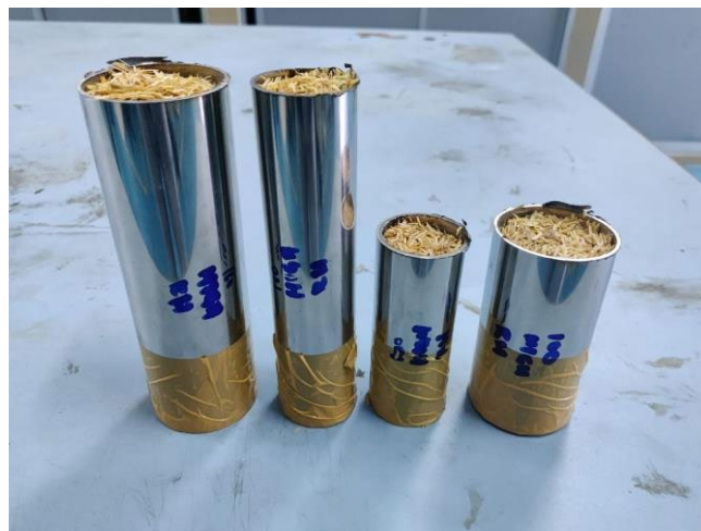
Figure 1: Stainless steel tubes filled with rice husk.
