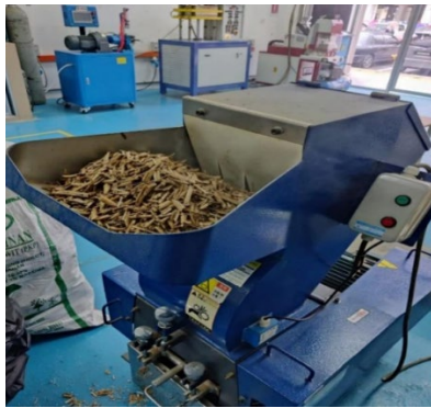
Process of crushing the kenaf fiber using a crusher machine.
