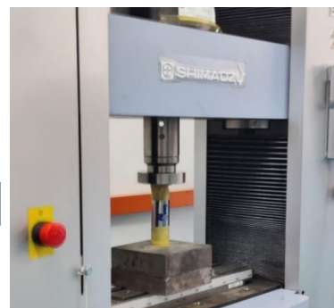
Conduct compression test using UTM Machine.
