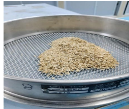
Process of filtering kenaf into the desired size.
