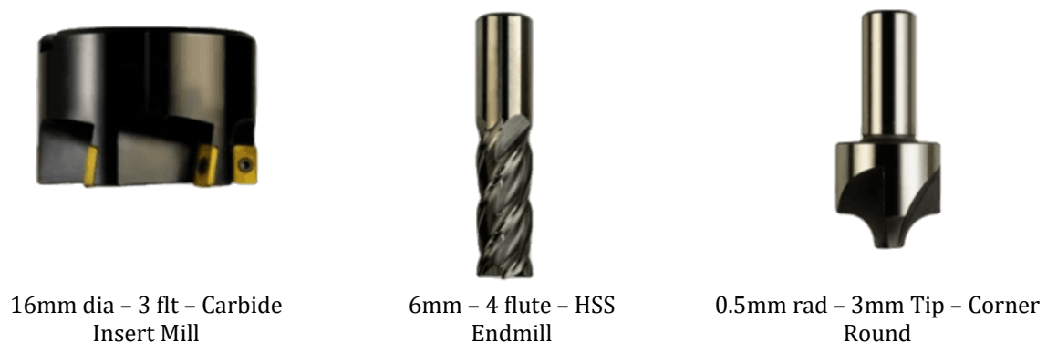
Figure 6: Tool selection in CAM.
