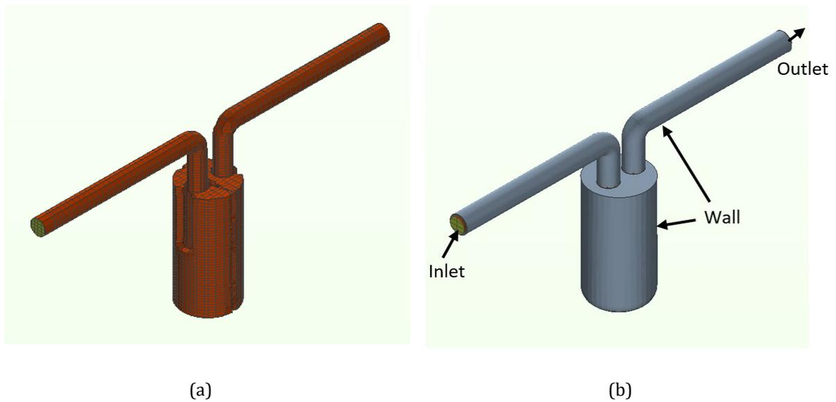
**Figure 3:** (a) Hex-dominant meshed model and (b) boundary conditions.
