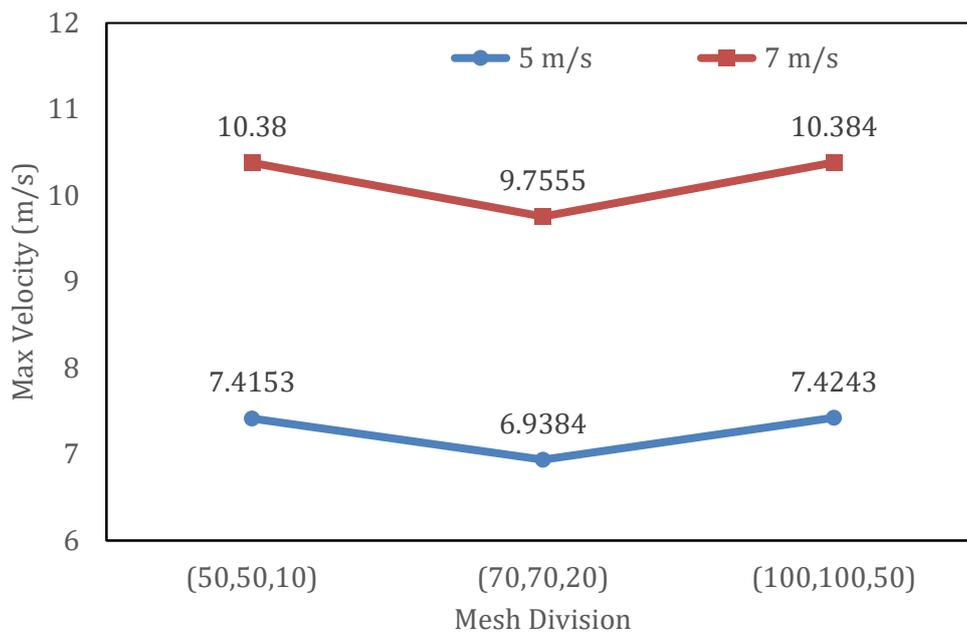
**Figure 5:** Maximum velocity for different mesh divisions at 5 and 7 m/s inlet velocity.
