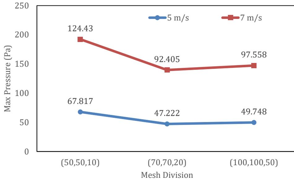
**Figure 4:** Maximum Pressure for different mesh divisions at 5 and 7 m/s inlet velocity.
