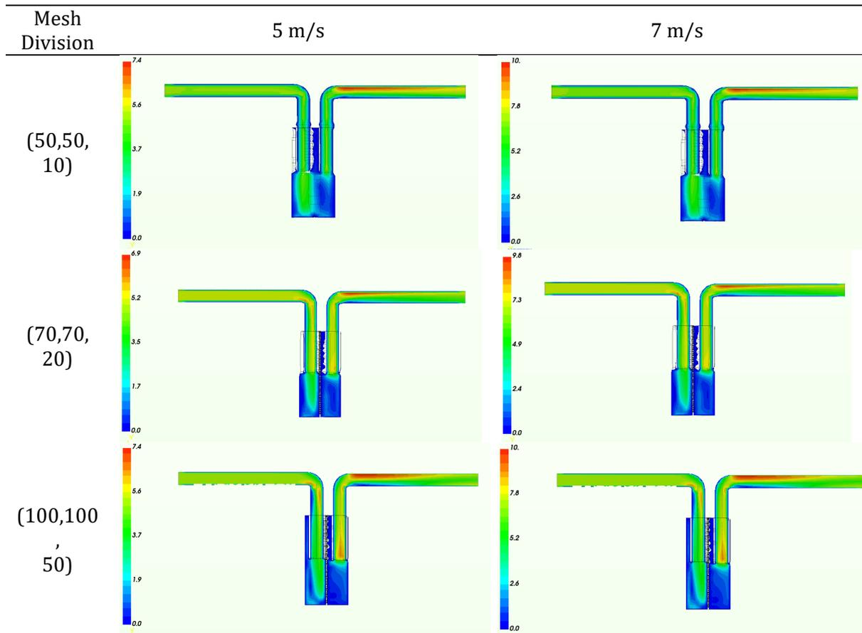
**Figure 7:** Velocity contour inside the hydraulic filter.
