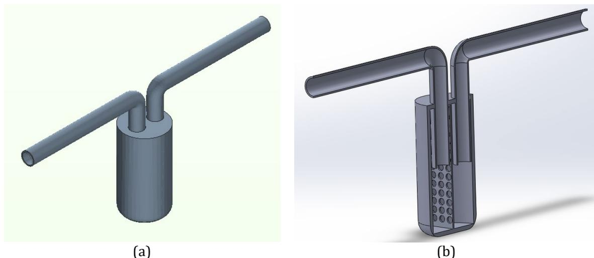
**Figure 1:** (a) 3D model of aircraft hydraulic filter and (b) cross-section view in SolidWorks.
