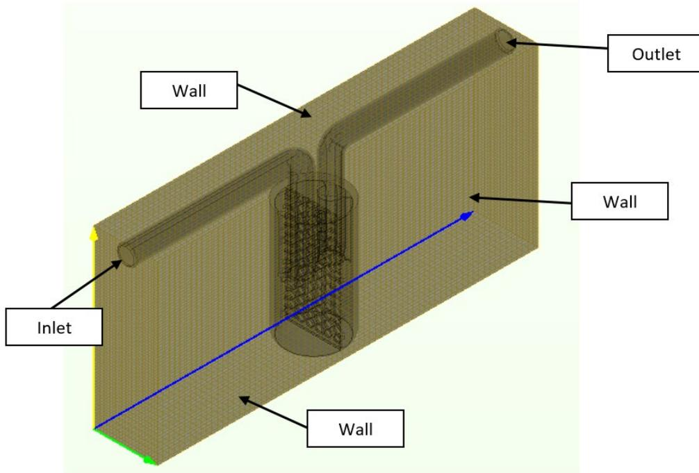
**Figure 2:** Hex meshing and boundary conditions defined prior to meshing of the aircraft hydraulic filter.
