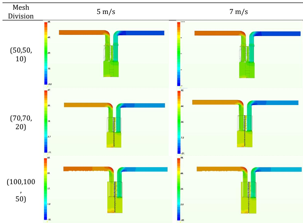
**Figure 6:** Pressure contour inside the hydraulic filter.
