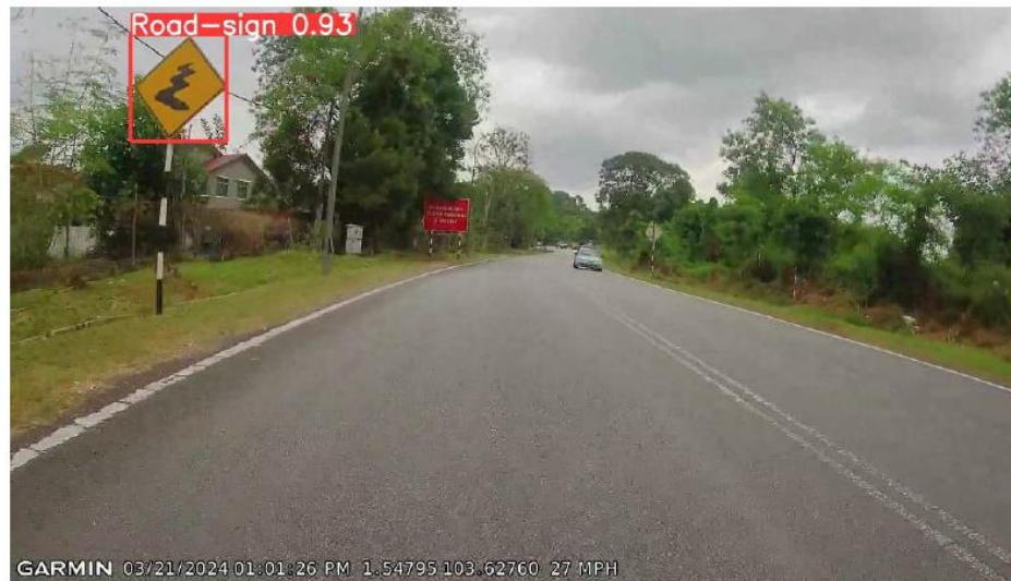
Figure 8: Road sign detection
