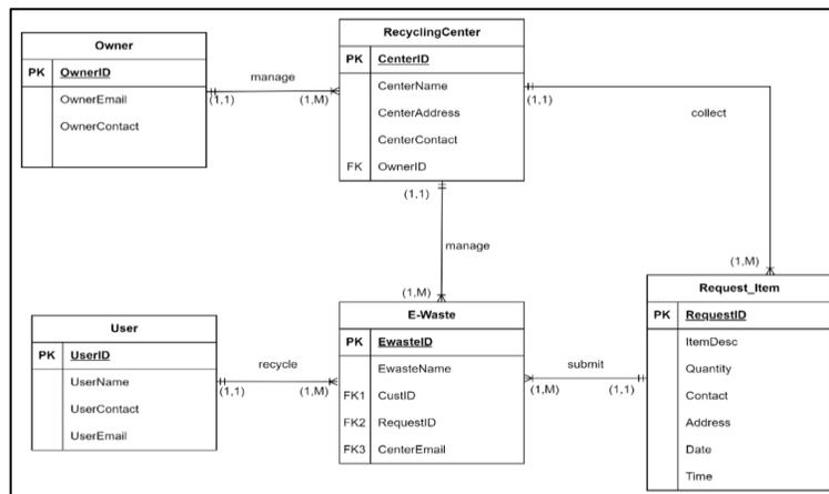
Figure 2: Entity Relationship Diagram of Project Application
