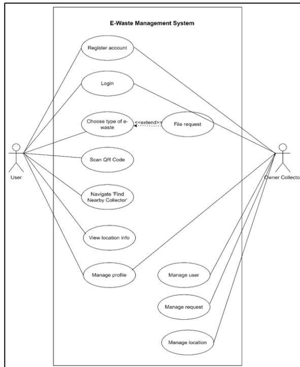
Figure 3: Use Case Diagram of Project Application
